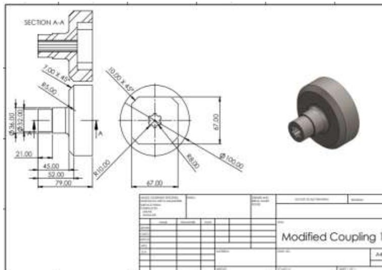
Figure 6: Solidworks Drawing of Modified Coupling Assembly (Male)
