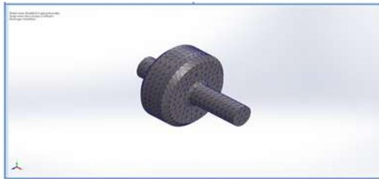
Figure 2: Mesh Model of Modified Coupler
