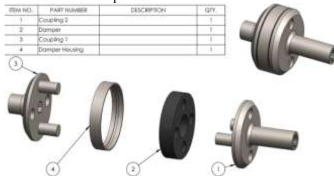
Figure 1: Exploded View of Modified Coupler
