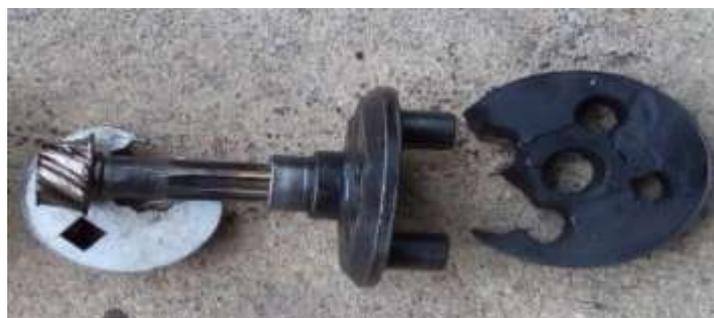
Plate III; Pinion, coupling and rubber damper.
