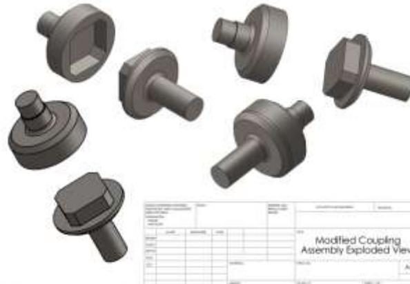
Figure 8: Solidworks Exploded View of Modified Coupler
