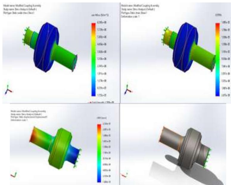
Figure 9: Stress Analysis of Modified Coupler.
