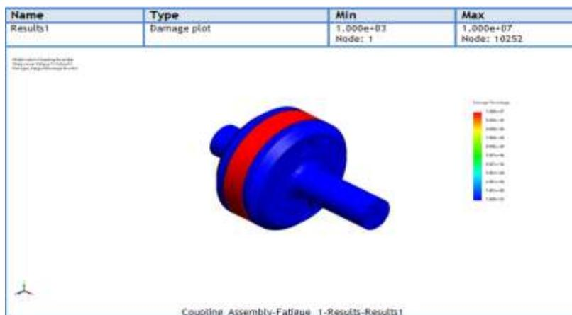
**Figure 4: Damage Analysis of Existing Coupler**
