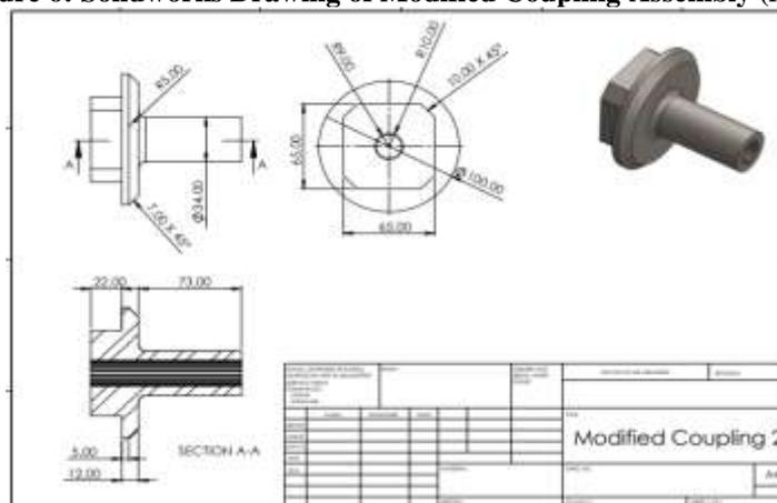
Figure 7: Solidworks Drawing of Modified Coupling Assembly (Female)
