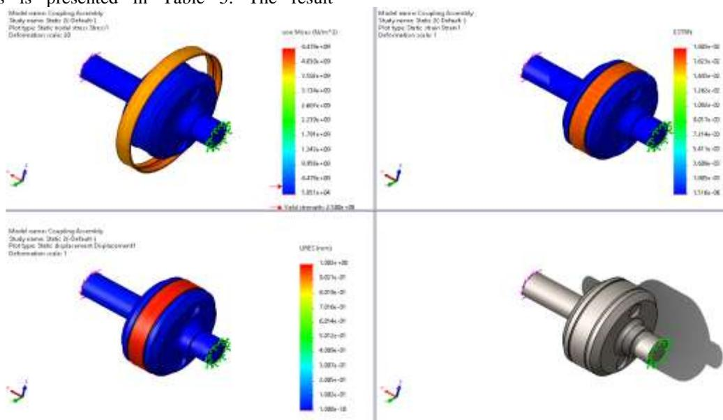
Figure 3: Stress Analysis of Existing Coupler
